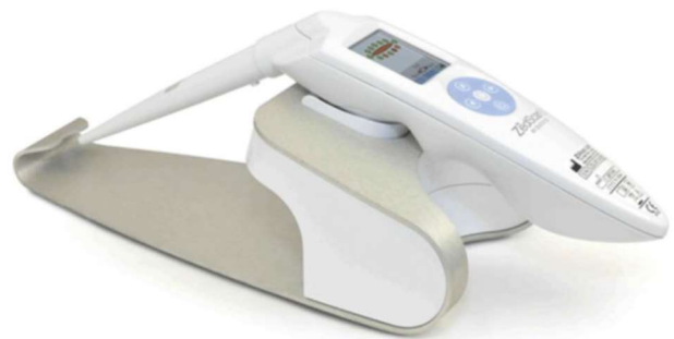
Fig. 1. The ZedScan™ handset for making the EIS measurements used in this paper. The handset is shown placed on the base
