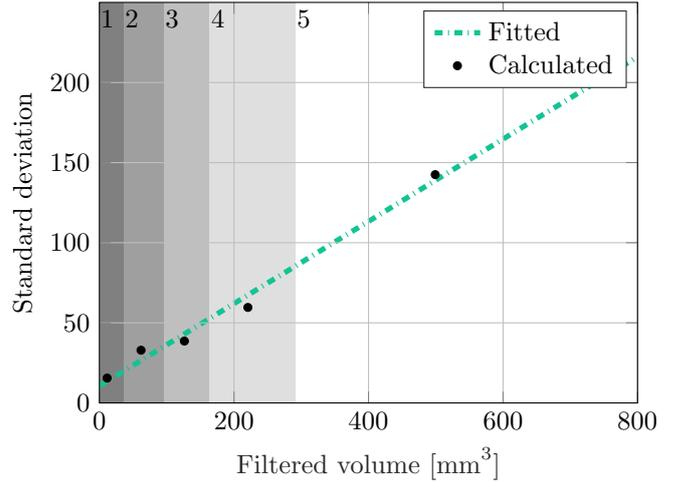
Fig. 4. Fitted noise model and the comparison of the distributions. Numbers (1-5) corresponds to the shaded regions, in which the standard deviation is calculated.
