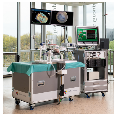
Fig. 1. A picture of the Cardiac Biosimulator platform showing the simulated environment (middle), endoscopic visualization of the valves (top) and visualization of pressures and flow (right).
