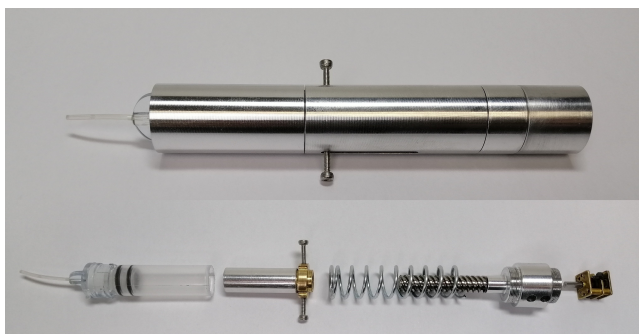
Fig. 4. Housing and drive mechanism of the mechanical insulin pump prototype
